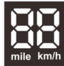
Speed Display Area Unit: MPH, KM/H The speed signal is taken from the Hall signal in the motor and sent to the instrument by the controller.(The time of a single Hall cycle, unit: 1MS) The meter will calculate the true speed according to the wheel diameter and signal data (the motor Hall also needs to set the number of magnets)
